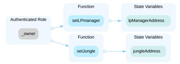
In the contract Vault the role jungleAddress has authority over the functions shown in the diagram below. Any compromise to the jungleAddress account may allow the hacker to take advantage of this authority and transfer in/out JUSD to/from the vault.
